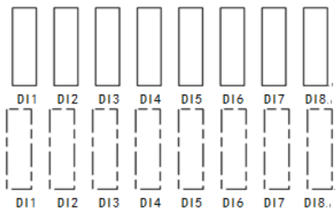
Figure 6-13 Status of digital input terminals
