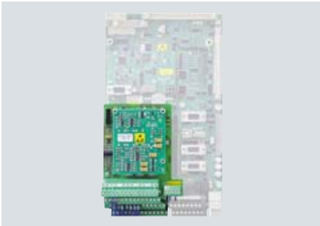
G05 Peripheral board 4 in the cabinet unit
