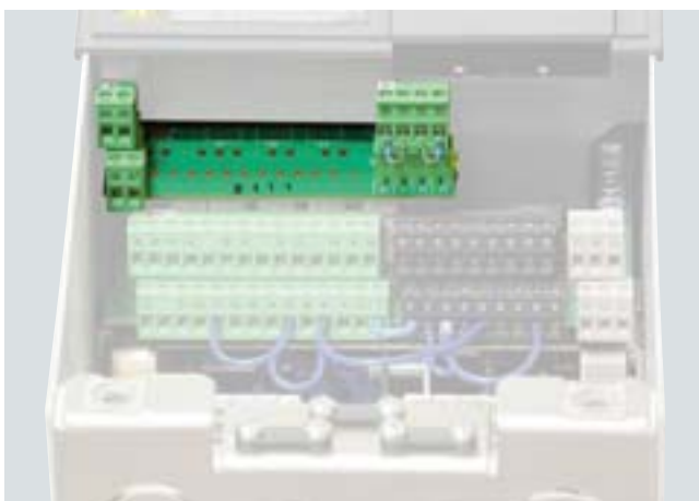
G03 Peripheral board 2 in the compact unit
